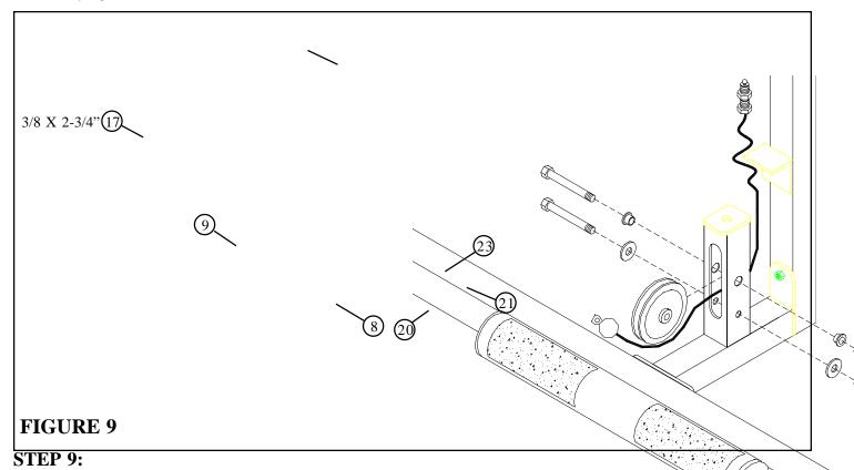
• Loop the ball end of the LOW ROW CABLE (12) around one 4-1/2" PULLEY (9) and SECURELY assemble the 4 (2" PULLEY (9) to the LOW PULLEY HOUSING (8) using two 3/8 X 2-3/4" BOLTS (17), two 3/8" FLANGE SPACERS (22), two 3/8" WASHERS (20), and two 3/8" LOCKNUTS (21). (NOTE: Make sure CABLE is routed between the PULLEY and the retaining bolt as shown in FIGURE 9.)
